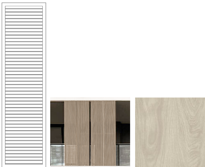
SCR1 | L04 Fixed Screen Aluminium, Rectangular Sections Pale Timber-look Finish
